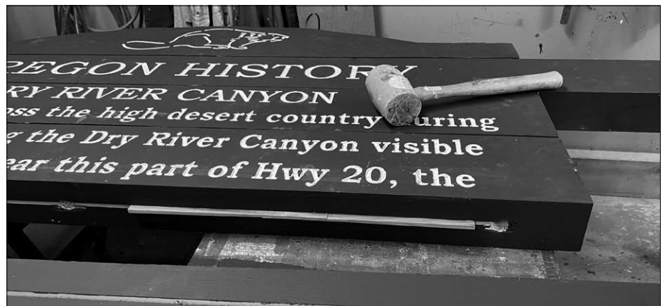
4) Spline Joints: Volunteers place splines between each board to reduce warping as the wood weathers in the elements.
