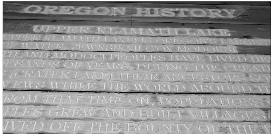
3) Painting: The wood returns to the Salem town shop where volunteers apply 6-8 layers of white paint in the letters and later roll-on Oxford brown paint.
