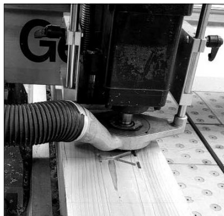
2) Routing: Text and the iconic beaver are routed into the boards at the ODOT sign shop.
