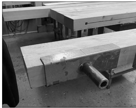
1) Wood Prep: Four-inch thick, rough-cut lumber is dried onsite for a year. Planks are planed to consistent 8- and 10-inch widths. Salem town then sands and uses a jig to predrill holes.
