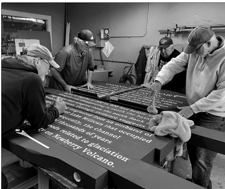
5) Assembly: All 9 boards get cinched together like a puzzle, then fastened with all thread rods.
