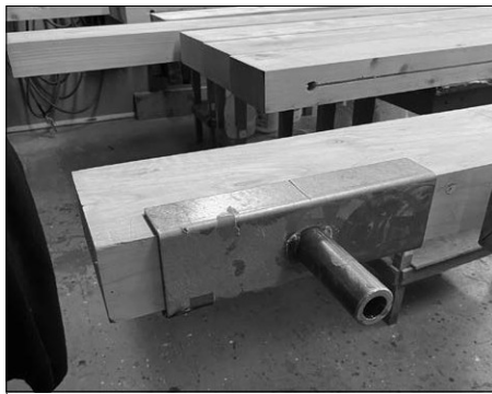
1) Wood Prep: Four-inch thick, rough-cut lumber is dried onsite for a year. Planks are planed to consistent 8- and 10-inch widths. Salem town then sands and uses a jig to predrill holes.
